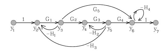
$$\frac{y_2}{y_1} = \frac{1 + G_3 H_2 + H_4 + G_3 H_2 H_4}{\triangle}$$
